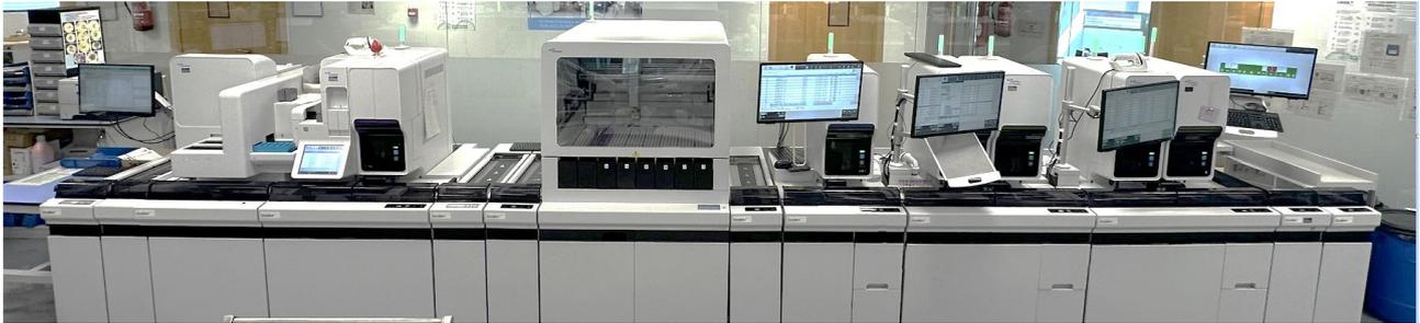
Fig. 15: Sysmex XN-9100 chain composed of, from right to left, 3 XN-10 analyzers; 2 XN-20 analyzers; a TS distributor; 1 SP-50 extender-stainer and a Cellavision® DI-60
